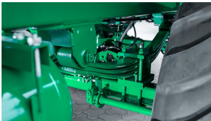
Composite chassis comprising 4 parabolic suspension springs for stable handling and a high level of comfort.
