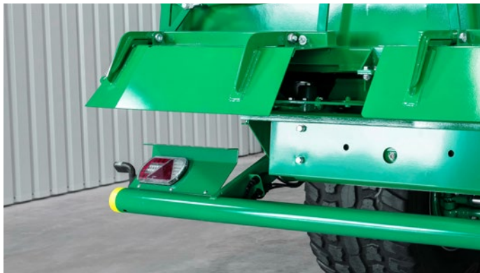
The boundary spreader device allows compact and precise manoeuvring along the edge of the field. It offers protection for other traffic users, prevents the spread material from entering waters and helps to counter under-fertilization of the edge of the field.
